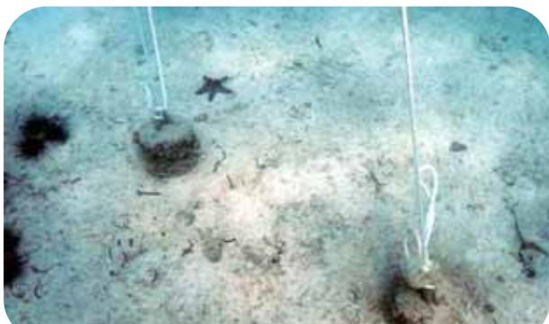
Two c. 25 kg concrete sinkers anchoring two corners of a 1.2 m x 5 m lagoonal floating nursery at Chumbe Island, Zanzibar (J. Guest).
